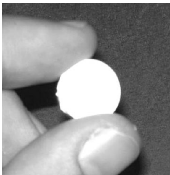
Figure 1 Image of a nonsupercritical microporous gel sample.
